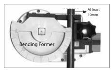
View the LCD screen and set to the desired angle by turning the Degree Selector Thumb Wheel.
