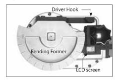
NOTE: Whenever the machine is **first plugged in** Press & hold the trigger of switch , it will automatically return to its (zero degree) starting position. in the other words the LCD screen shown (zero degree) The machine is now ready to perform the bending operation.
